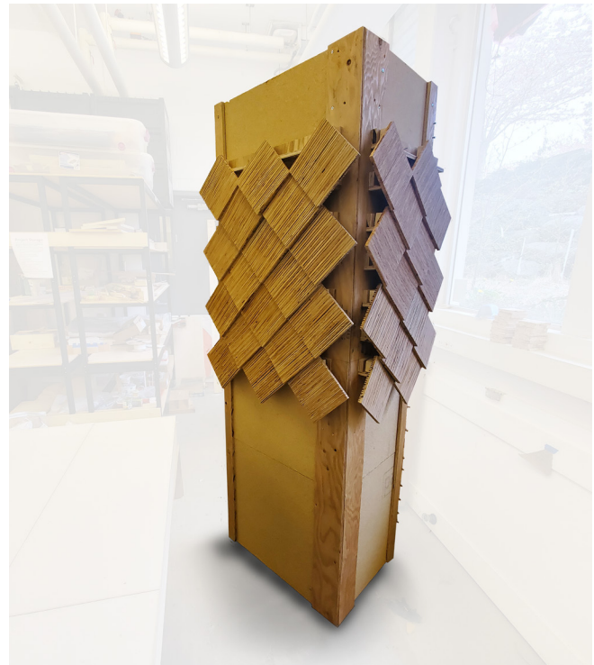
Figure 4. Mock-up of light-wood frame wall prototype. Author.
